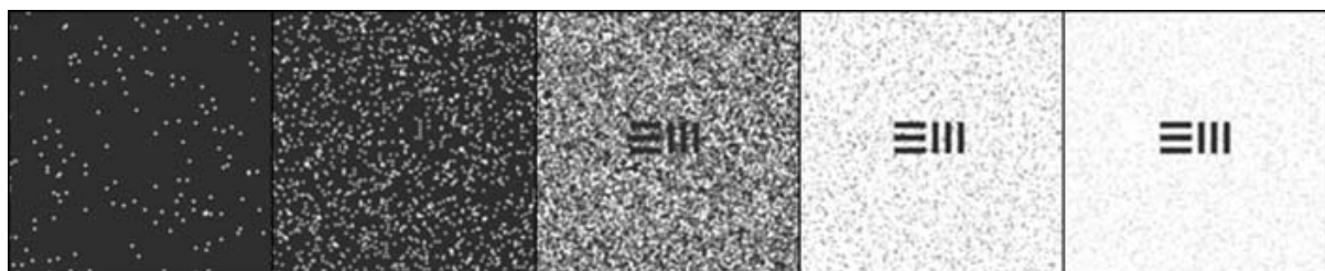
A simulated smaller target of approximately 60 lp/mm, intensified at various light levels
