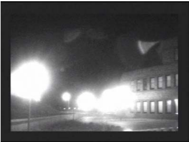
Example of halo experienced with GaAs Tubes
