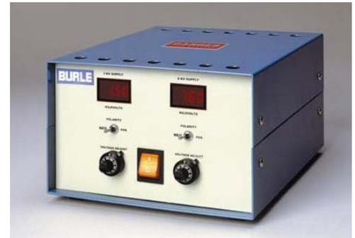
Model PF1054 is a solid-state, bench-top Dual High Voltage Power Supply that can provide DC outputs of up to 3 kV and 8 kV. The output polarity can be set to either negative or positive via a front panel switch. This model offers high precision and stability in a compact, economical package which makes it ideal for many laboratory applications.
