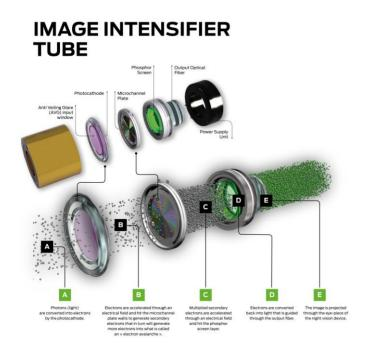
This is the key (engine) component of any night vision device.
