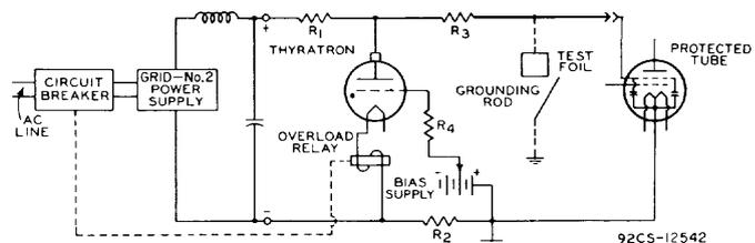
**Figure 4 - High-Speed Electronic Protective Device for Removing Grid-No.2 Voltage in the Event of Abnormal Operation**
