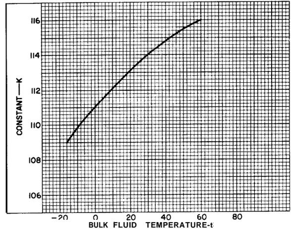
**Figure 6 - Determination of Constant for FC75 in Plate-Dissipation Calculation**
