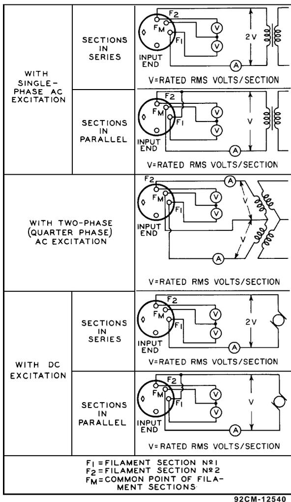
**Figure 5 - Filament Excitation Circuits for Beam Power Tetrodes Having 2-Section Filaments**
