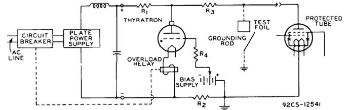
**Figure 2 - High-Speed Electronic Protective Device for Removing Anode Voltage in the Event of Abnormal Operation**
