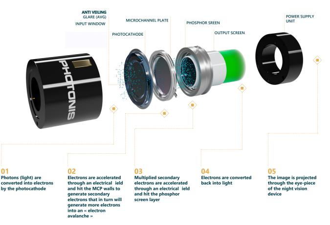
The MCP is a thin glass disc, less than a half a millimeter thick, which contains millions of small channels. When an electron coming from the photocathode strikes the inner wall of one channel, several secondary electrons are generated by the impact. Each of these secondary electrons will be accelerated
