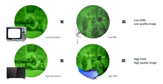
Together SNR x Resolution constitute the Figure of Merit (FOM): the difference in ranges for detection of an I<sup>2</sup> with 1600 FOM and 2400 FOM is marginal at night levels 1-3, but it is very significant at night levels 4-5 (the higher FOM results in more than 45% increase of the Detection, Recognition and Identification ranges).
