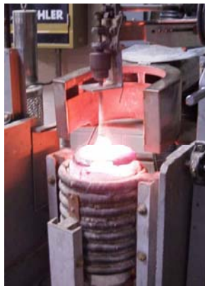
Small Batch Glass Making in Platinum Crucibles
